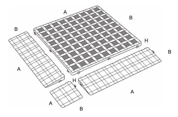
The modular Epsilon grating is insulating and easy to lay, thanks to the system hooking all various elements one to another. It enables the creation of antislip flooring in all sizes. Rated operational voltage 3 kV. Epsilon comes complete with a side and corner joint for even more functional floor paving.
