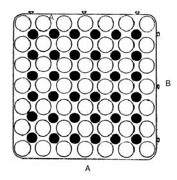
The self-modular Sigma elements made of special green shockproof resin are particularly suitable for flooring in graphic and mechanical industry as they can absorb to a great extent the vibrations produced by plants, and dampen the relevant noises. They are also an efficient solution in the galvanic industry thanks to their excellent resistance to acids and corrosive liquids. They stand pressure loads without yielding up to 680 kN per sq.m.
