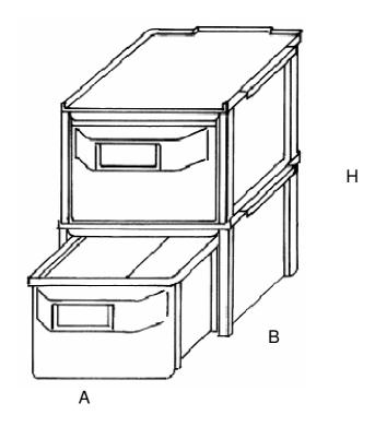
This lightweight self-supporting drawer unit is designed on the build-it-yourself principle for creating storeroom walls of any size. The drawers can be removed completely and stacked and are also available in a version resistant to oils, fats and solvents.
