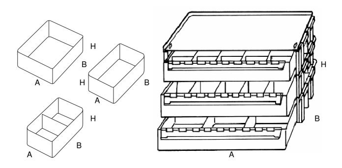
The basic module (casing and drawer) of this drawer unit can be used to build walls and partitions for storerooms, workshops and points of sale. Inside of drawers can be divided by the Beta bins, coming in 4 different sizes.
