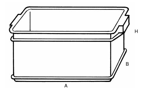
Stackable containers with side handles, suitable for small metal products and pharmaceuticals. Also available in non-toxic material for use with foodstuffs or in conductive material for electronic components.
