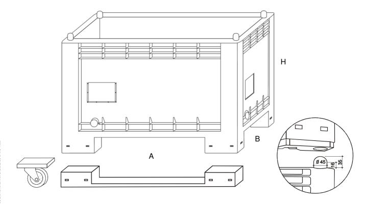
The CARGOPALLET 300 PLUS is versatile and robust, has good structural rigidity, resists deformation. Ideal for the textiles, pharmaceuticals, metallurgical, rubber treatment and plastics industries. The overlap of Cargopallet 300 Plus is secured by 4 cylinder/spherical pins obtained directly from the mold on top of the container that fit into appropriate seats machined at the bottom of the legs/runners of container.
