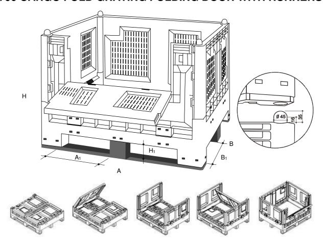
Cargo Fold 700 grating folding door with runners is completely folding. With this system, in case of transport and storage of empty containers, you shall earn 63% in volume: a stack of eight folded Cargo is the same height as three open ones.
