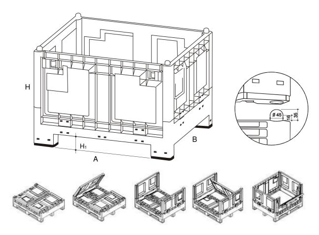
Cargo Fold 700, the first cargopallet with collapsible walls and available on wheels, is even more flexible and ready to meet transport and storage requirements. The special white polyamide wheels, fastened to the base of the Cargo Fold, include special galvanized steel cross bars to ensure hold and stability of the load; moreover they allow use with heavy duty loads up to 600 Kg.
