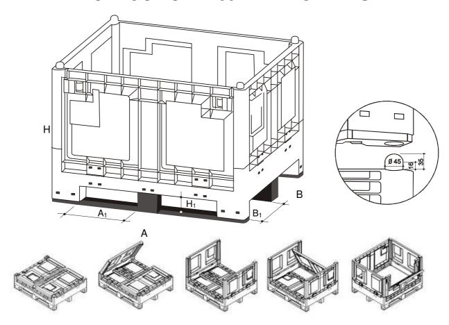
Cargo Fold 700 with runners is completely folding. With this system, in case of transport and storage of empty containers, you shall earn 63% in volume: a stack of eight folded Cargo is the same height as three open ones.
