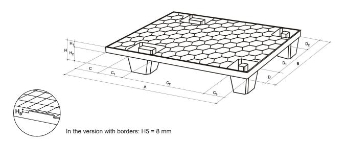
The Pallet My-A series is now complete with the 400x600 measure, ¼ of the standard European size. The feet are deliberately asymmetric to allow the use with forklift. Thanks to the honeycomb structure the Pallets My-A are very strong.
